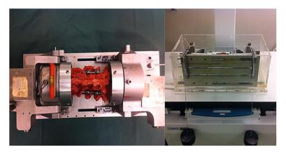
**Figure 1.**The experimental setup is shown from above (left) and side (right) with lumbar spinal specimen (L1-L5) positioned in the four-point bending device and preloading weights.
